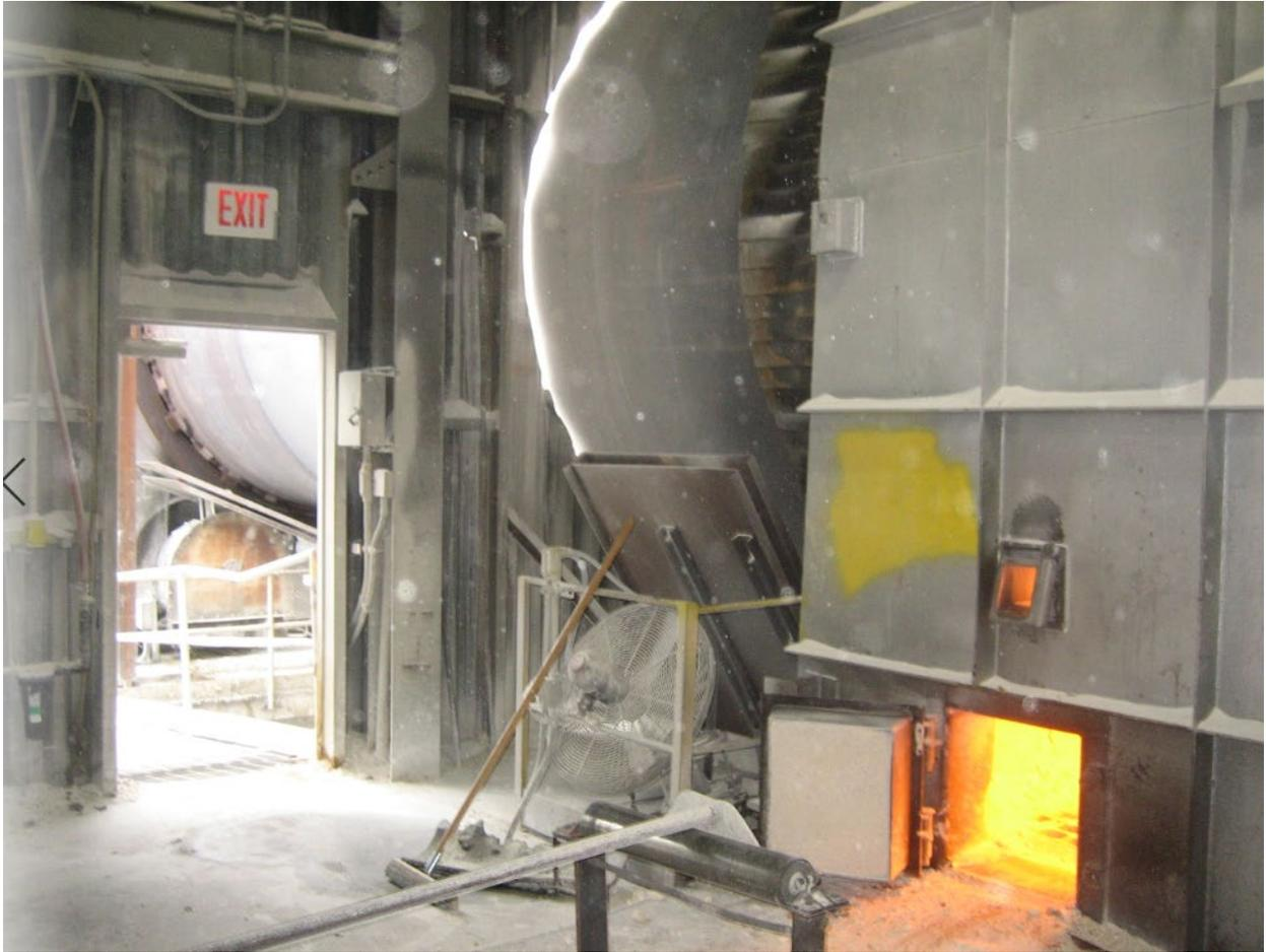
Figure 2: Alternative view of horizontal rotary kiln used to make Lime.
