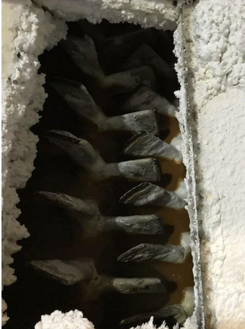
Figure 4: Slaking chamber where Lime and water are mixed with paddles at a constant temperature.
