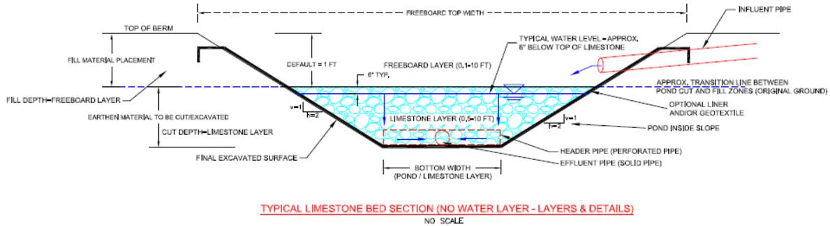
Figure 3: Typical Cross Section View of a Limestone Bed (LB) without a water layer.
