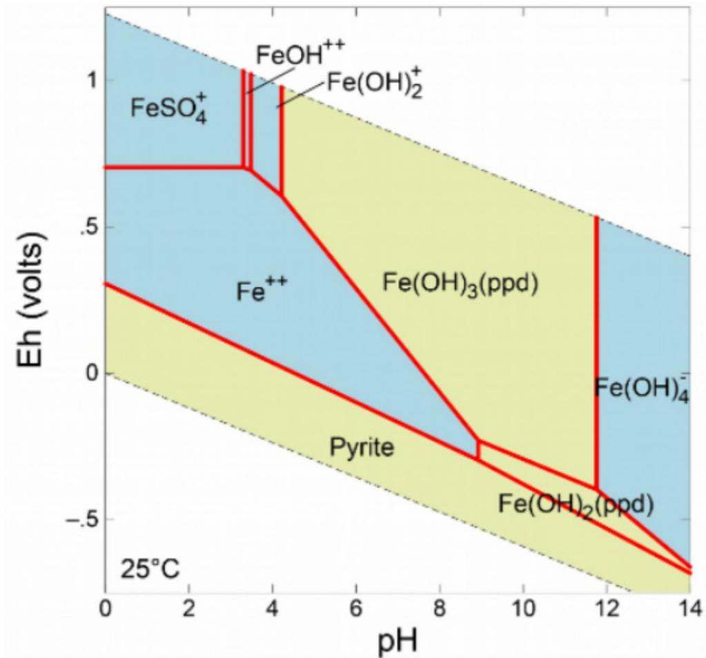
Figure 12. Fe(OH)<sub>3</sub> solubility diagram with pH versus Eh. If water in the limestone layer contains any oxygen, ferrous iron will oxidize and precipitate as the pH increases > 6.0.
