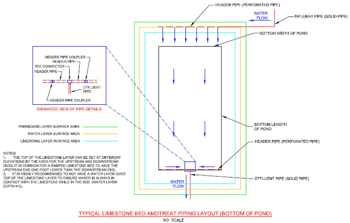
Figure 4: Plan View of the Limestone Bed (LB) to Illustrate Common Piping Layout and Components (Used in AMDTreat Piping Calculator) and the Layer Surface Areas
