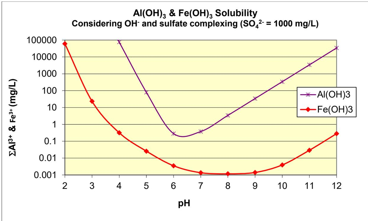
Figure 11: Aluminum becomes insoluble at pH > 5.5 and will precipitate and accumulate in the limestone. Ferric iron becomes insoluble at pH > 4.0.
