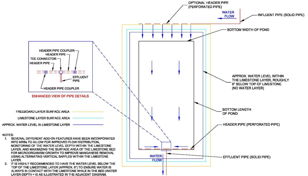
Figure 3: Diagram showing the default influent and effluent piping scheme used in AMDTreat for a MRB.
