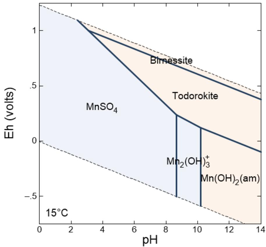
Figure 9: Pourbaix diagram illustrating manganese stability at various Eh/pH conditions.
