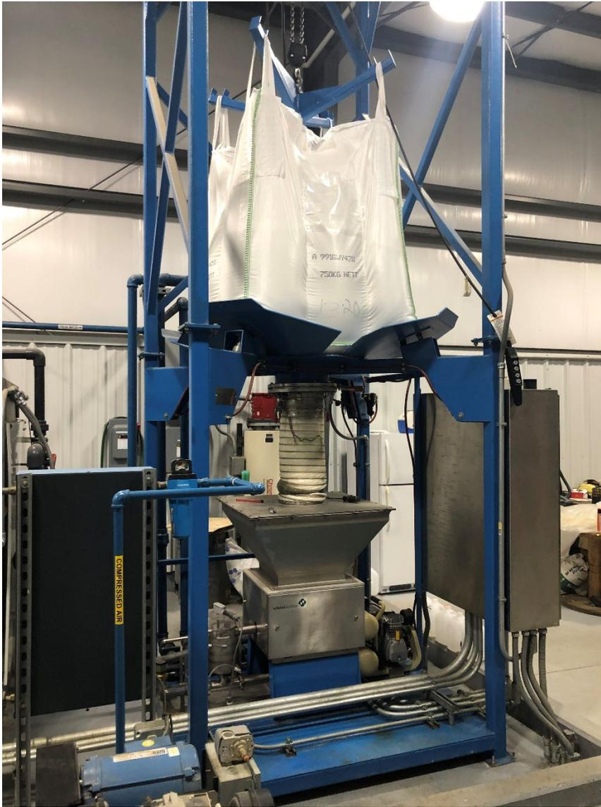
Figure 3. Super sack (1,650 lbs) feeder option as part of an automatic dry polymer make down system that automatically dispenses dry polymer product to produce a made down solution.
