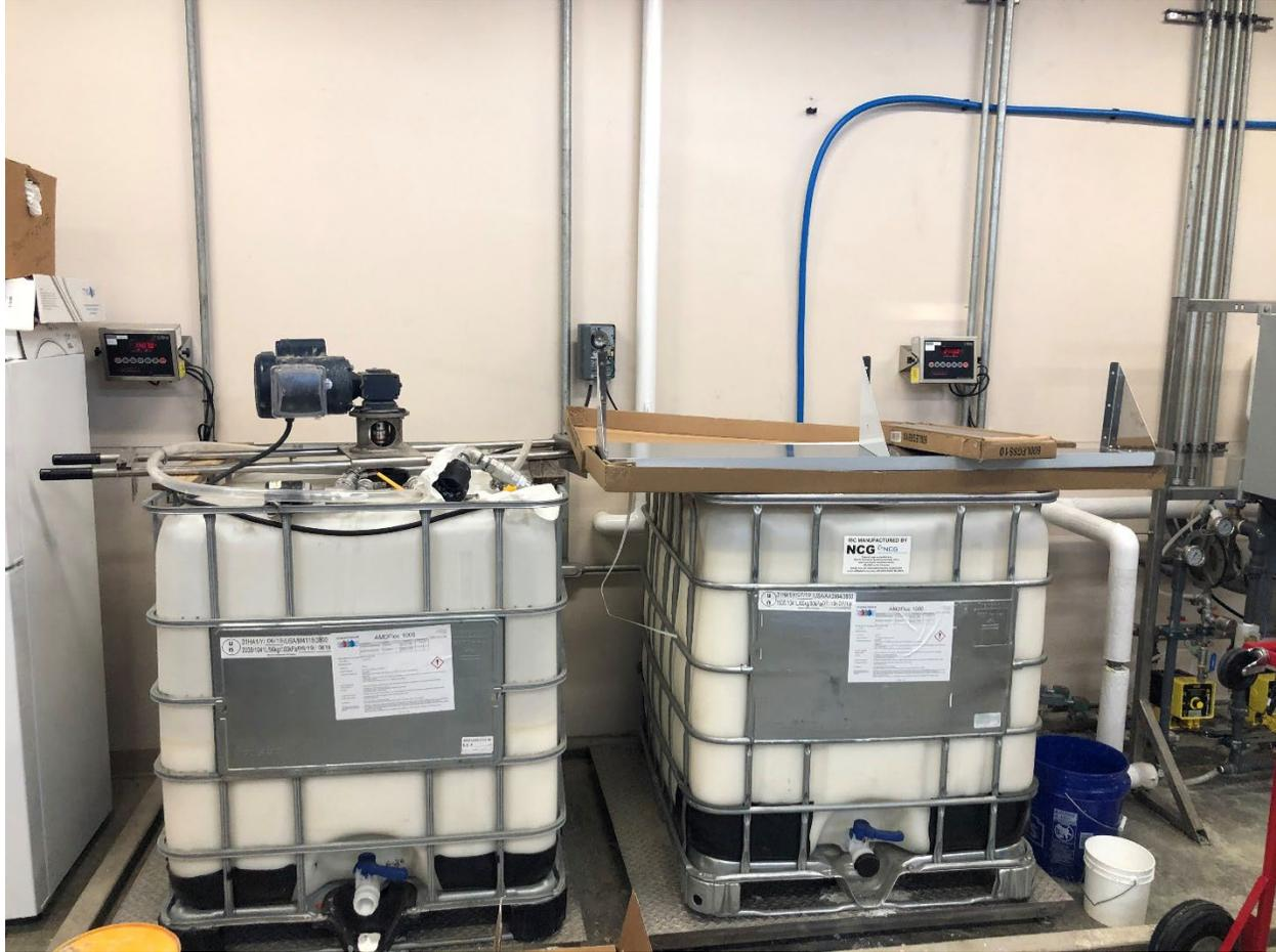
Figure 2. Emulsion polymer totes (275-gallon) for use at a mine drainage treatment facility in Pennsylvania.
