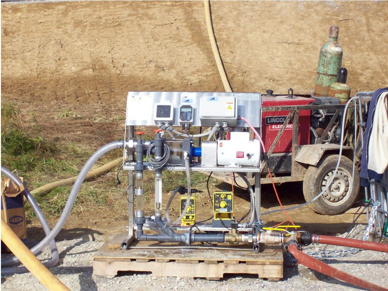
Figure 1: Blending skid with progressive cavity pump and computerized controls for emulsion polymer used at a site for flocculating iron hydroxide sludge and dewatering in Geotubes.
