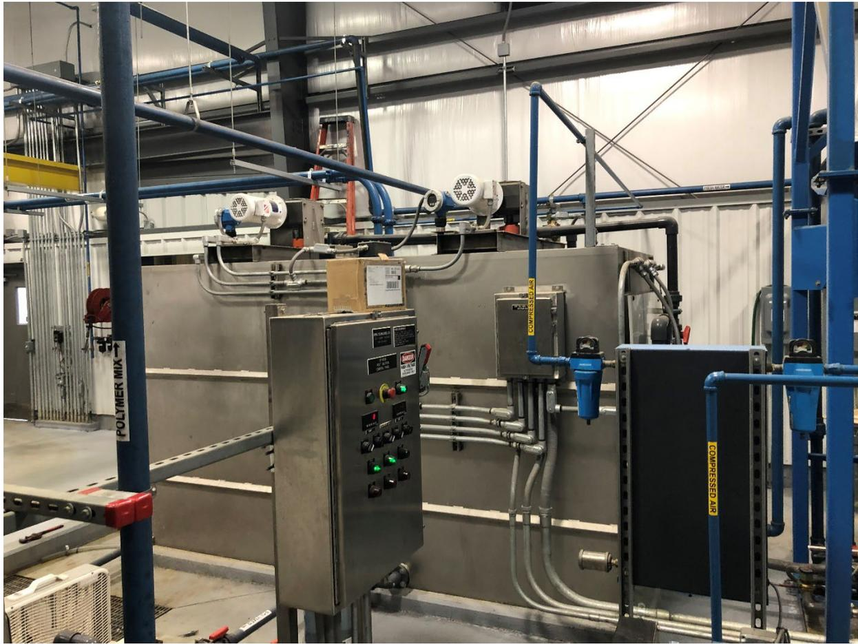
Figure 5. Stainless steel blending/aging tank for made down dry polymer solution with mixers mounted over the tanks.
