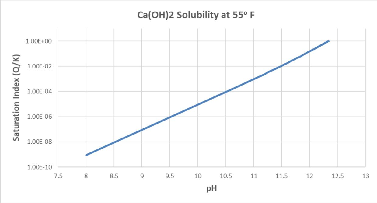
Figure 1: Graph showing saturated solution of Ca(OH)<sub>2</sub> is achieved at a pH of 12.4 at 55 °F.
