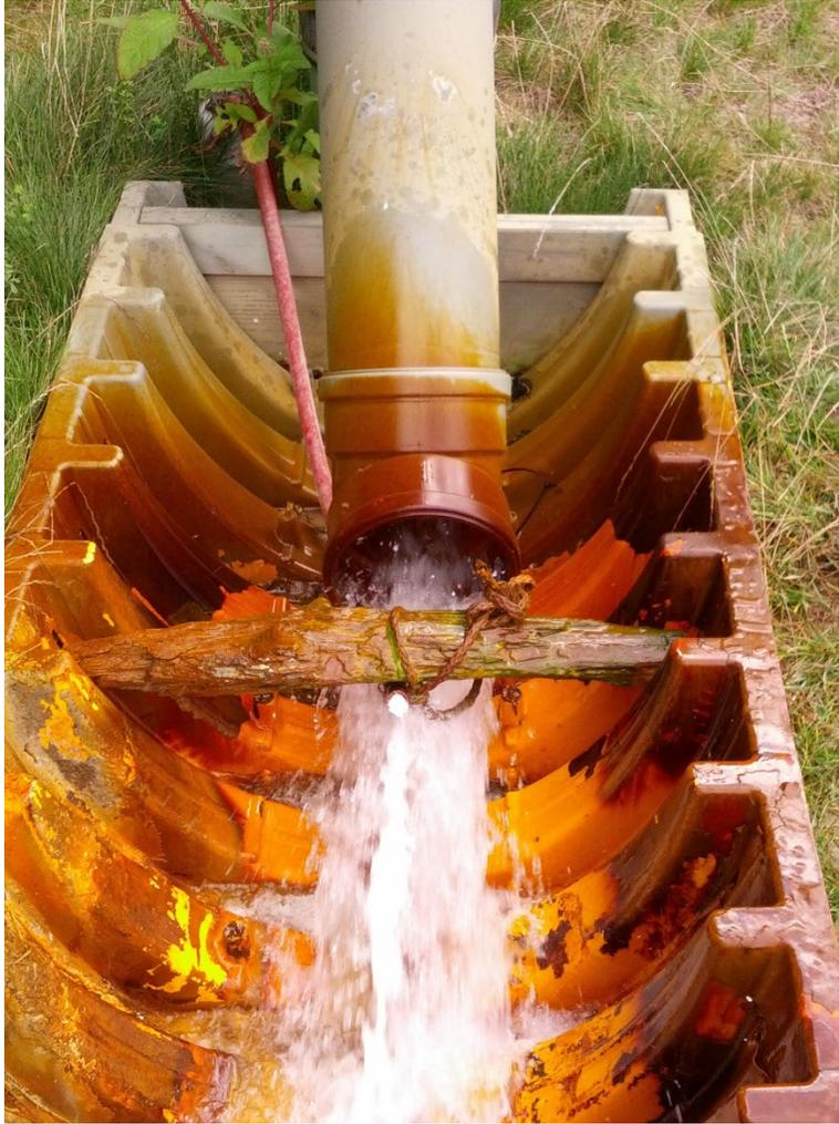
Figure 9: Lime Slurry (small red rubber tube) introduced to mine water in a mixing channel.
