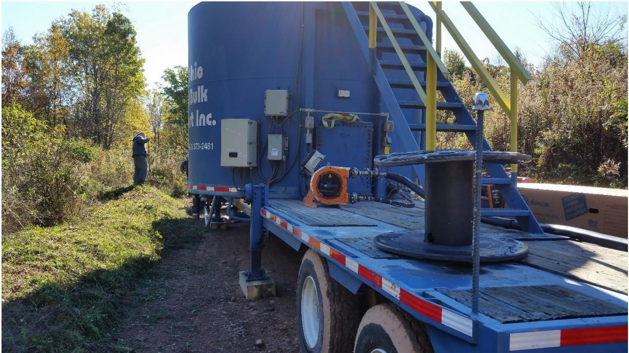
Figure 3: Portable lime slurry system in use at a PA Anthracite AML Discharge (Quakake Tunnel Discharge) to evaluate watershed impacts in consideration of a full scale permanent
