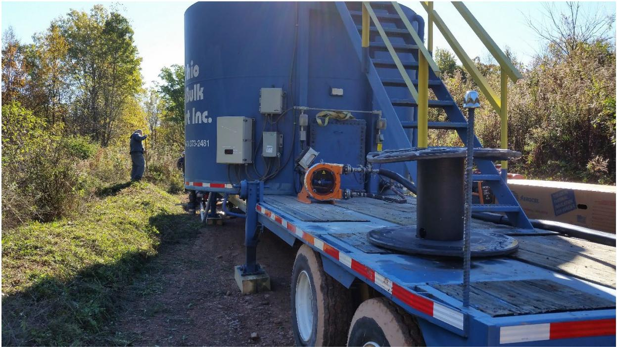
Figure 3: Portable lime slurry system in use at a PA Anthracite AML Discharge (Quakake Tunnel Discharge) to evaluate watershed impacts in consideration of a full scale permanent
