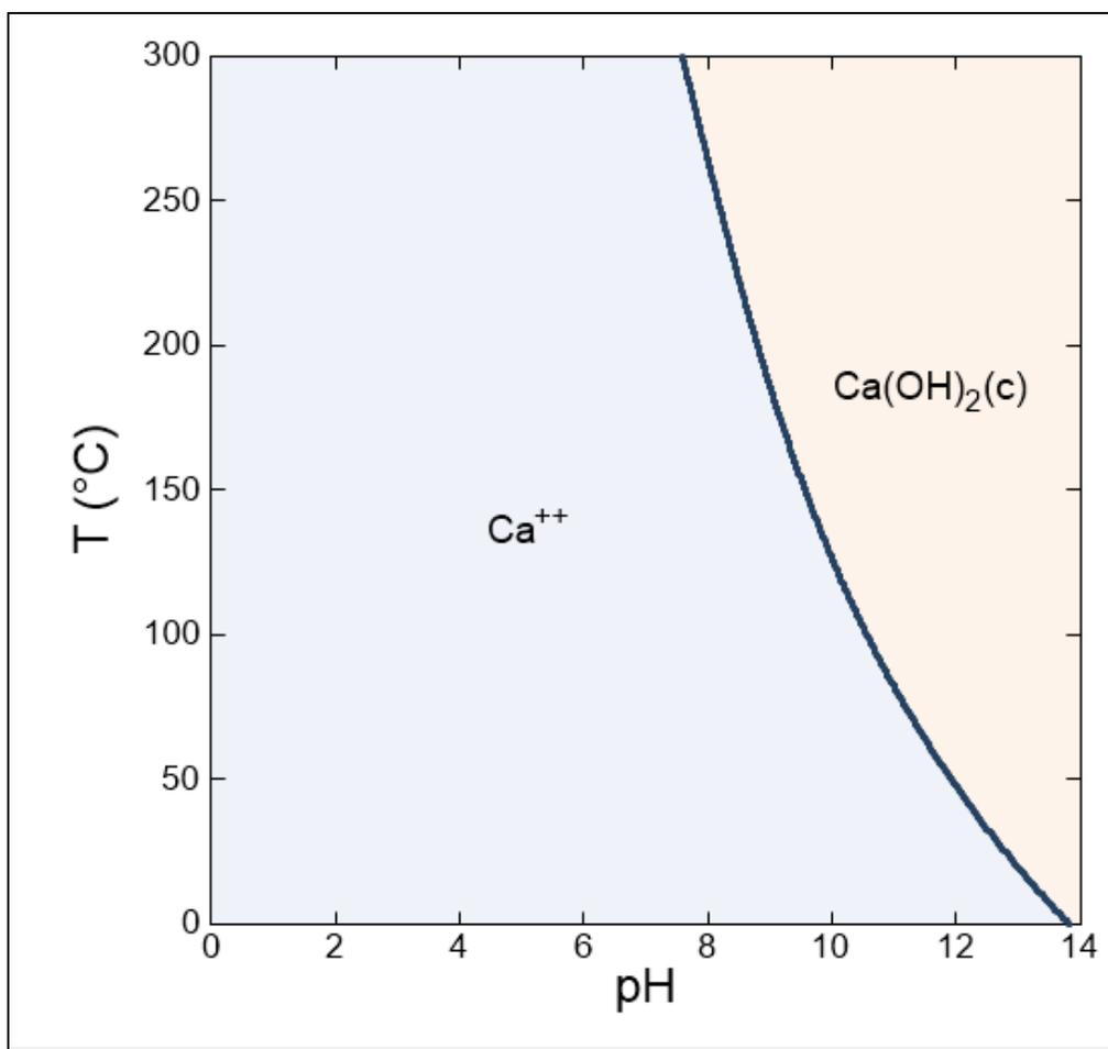
Figure 2: Graph showing the inverse relationship between solution temperature, pH, and solubility of  $\text{Ca(OH)}_2$ .
