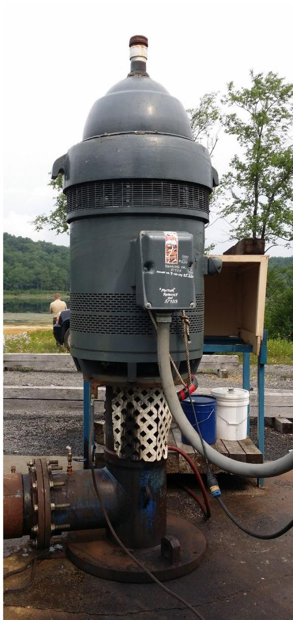
Figure 1. Vertical Turbine Pump at a mine site in West Virginia used to pump water from an underground mine pool to the surface for treatment at an active chemical treatment facility.
