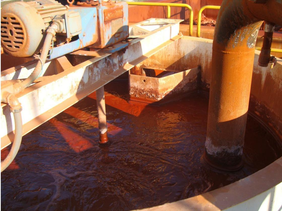
Figure 6: Mechanical mixer in a welded steel CSTR Reaction Tank.
