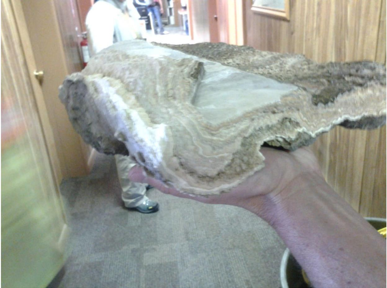
Figure 3: Photo of calcite and gypsum scale that can develop in highly mineralized mine water. Annual O&M cost calculations must account for this situation.
