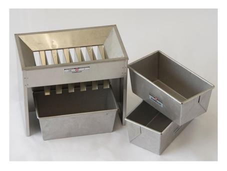
This 14-inch-long stainless steel sample splitter has a removable hopper constructed of 12 chutes that discharge alternately to front and back. Chutes are ¾ inch wide. Two pairs of cold-rolled steel pans come with the unit.
