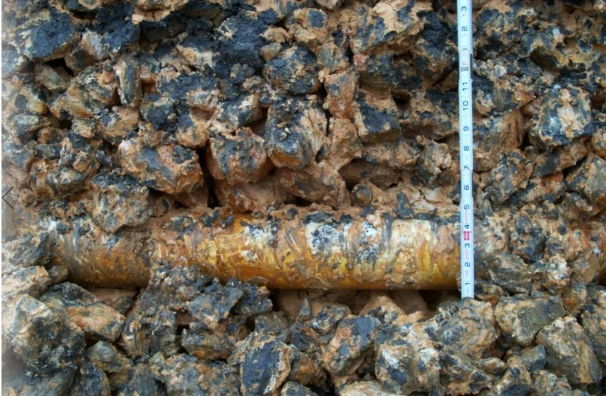
Figure 14. Whiteish aluminum hydroxide sludge accumulating within the Limestone layer due to the increase in pH. Note the flush pipe had little effect on preserving the porosity near the pipe.
