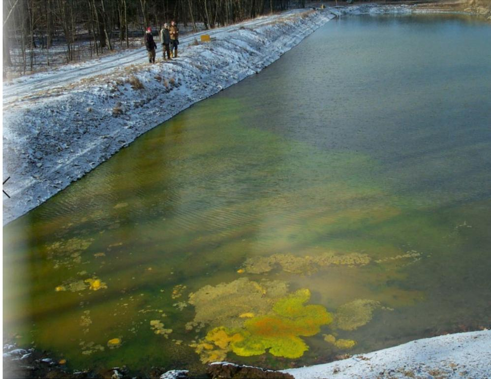
Figure 12. Rhodamine dye test to identify area where short circuiting is occurring. Dye was detected in the VFP effluent after 30 mins and the spread of the dye shown in photo remained constant for 8 hours indicating the location of the short circuit. This area was excavated and carefully rebuilt to eliminate the short circuit caused by poor construction practices.
