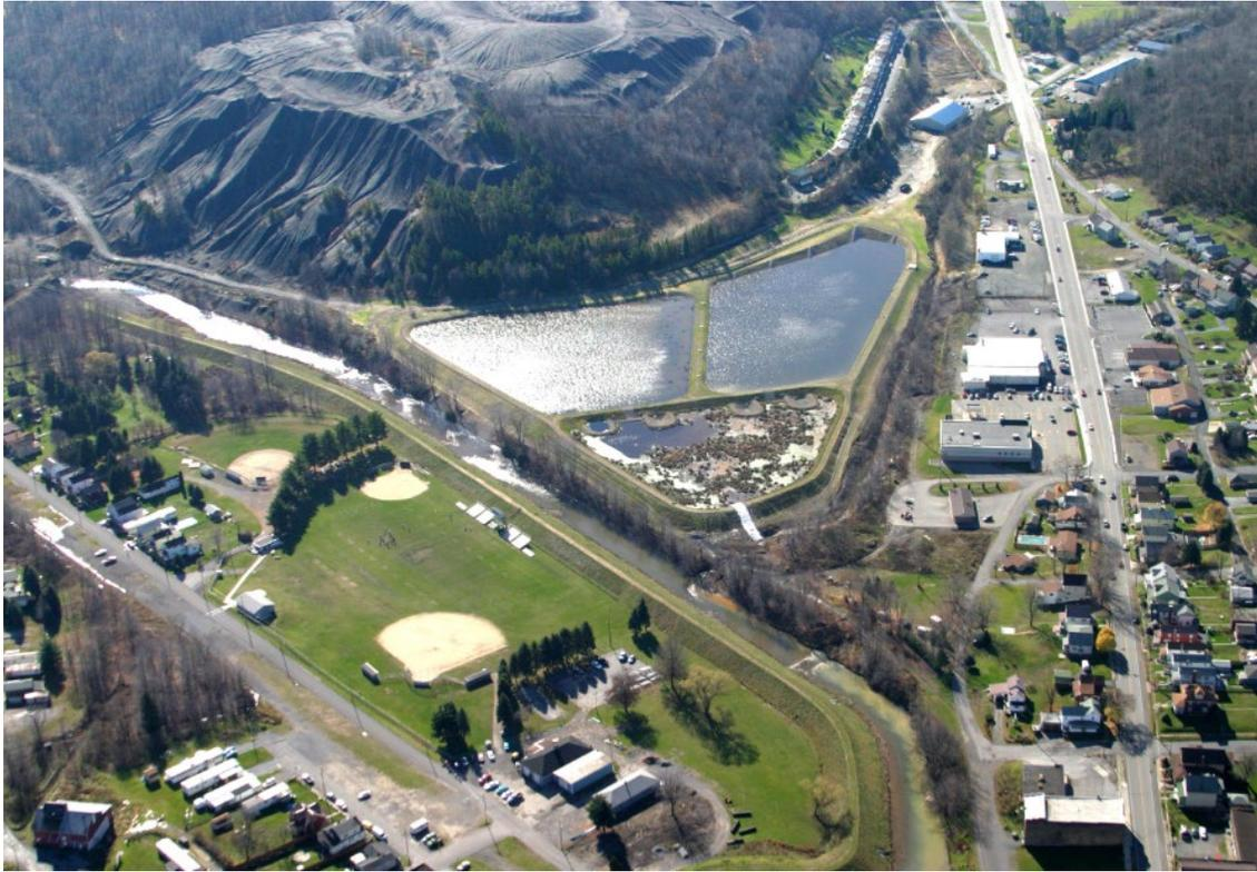
Figure 8. Two 2.5-acre vertical flow ponds flowing into a polishing wetland. Note the instream precipitation of metals caused by the alkaline effluent mixing with the acidic receiving stream.
