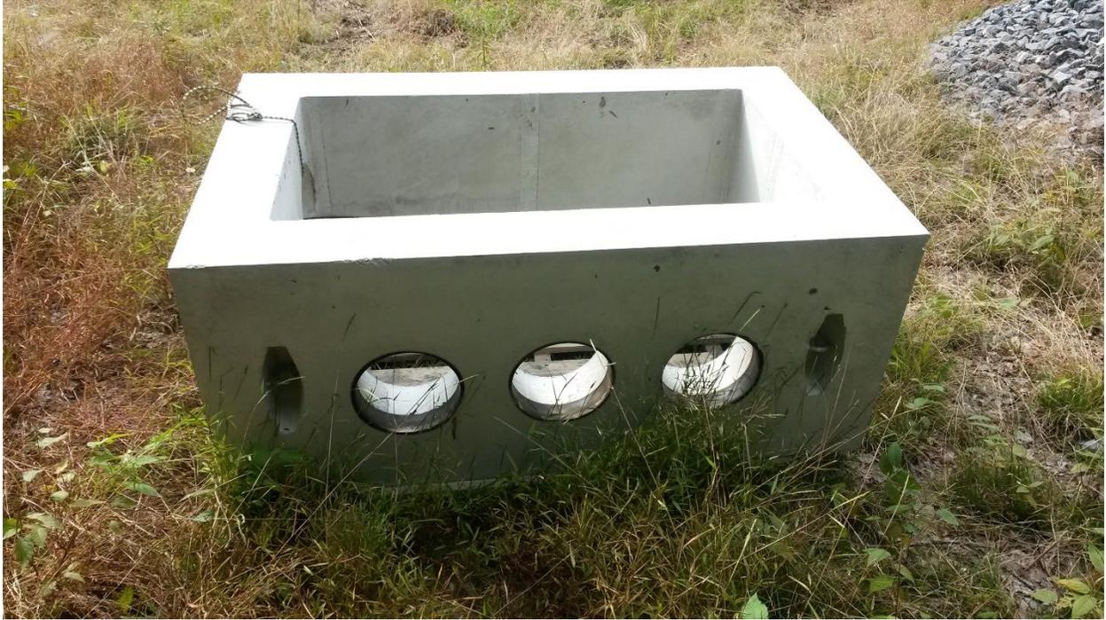
Figure 20 – Flow Splitter Box Prior to Installation. Pipe Gaskets are cast in place in precast yard.
