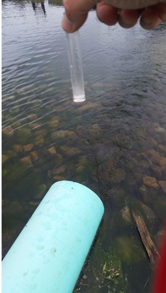
Figure 23: Effluent of 2-acre wetland receiving a suspended iron load of 60 lbs/day. The effluent iron concentration is less than 0.2 mg/L. Note lack of iron-stained rocks near effluent pipe and water clarity in water-filled tube.
