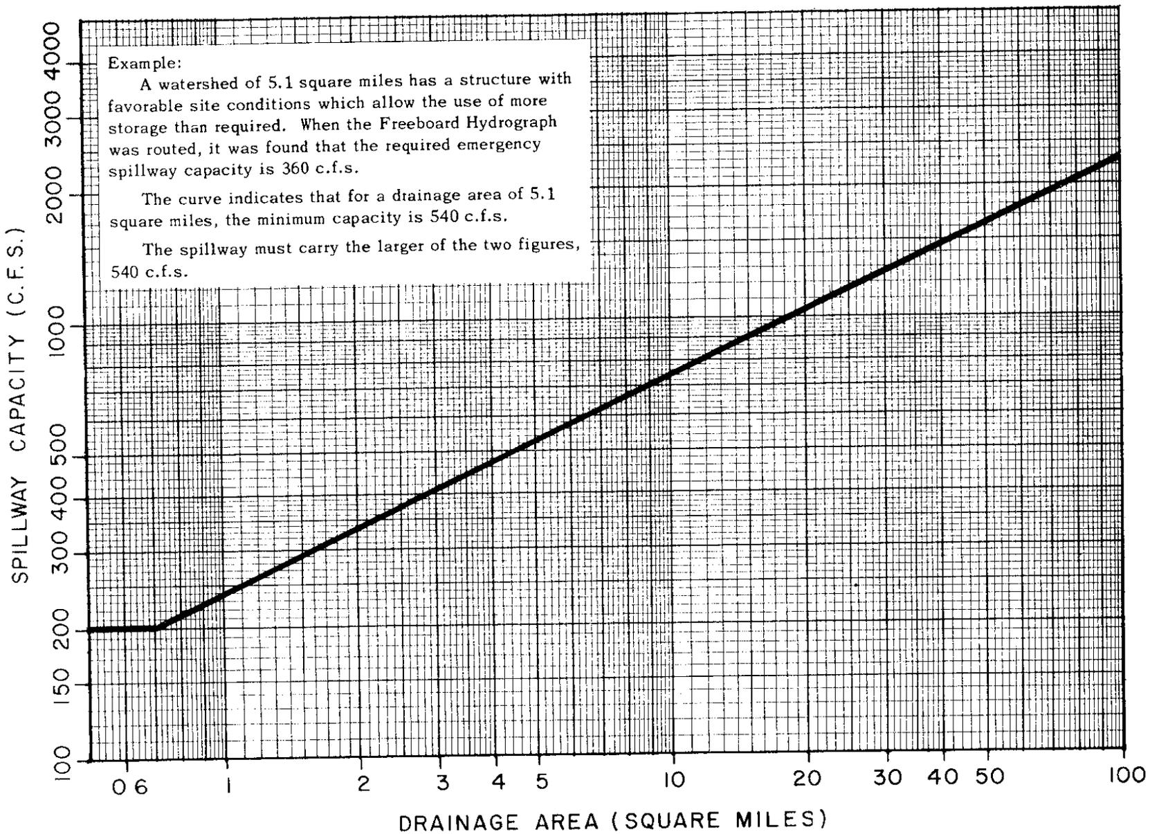
Minimum emergency spillway capacity - c.f.s.
