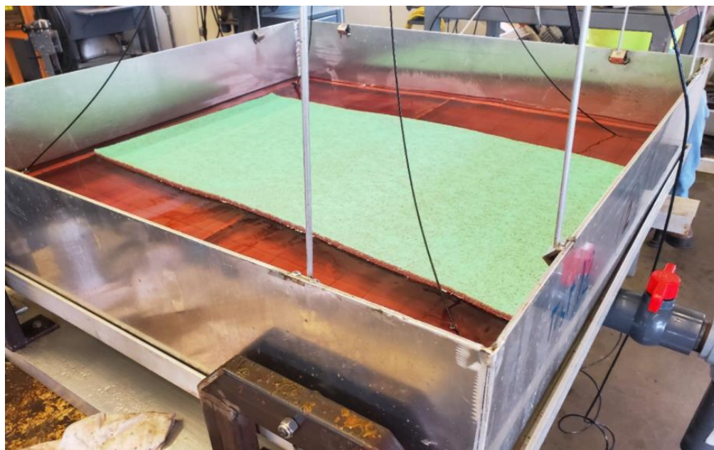
Figure 4 View of an open-cell foam sorbent sample undergoing testing
