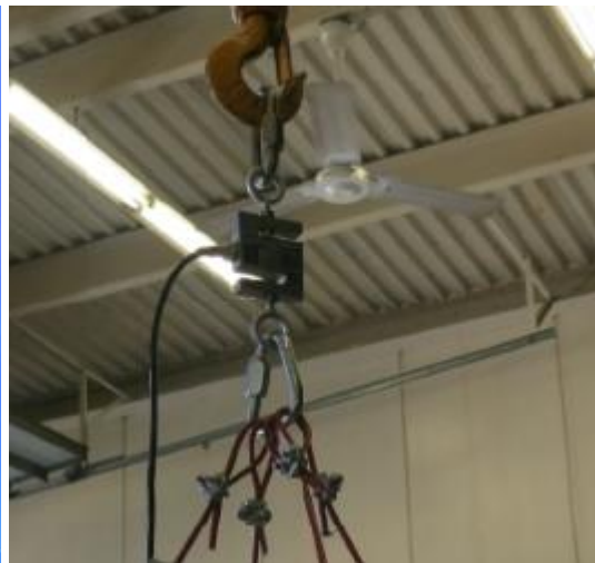
Figure 2 Screen showing load cell measurement in pounds (left) and Hoist-mounted load cell (right)
