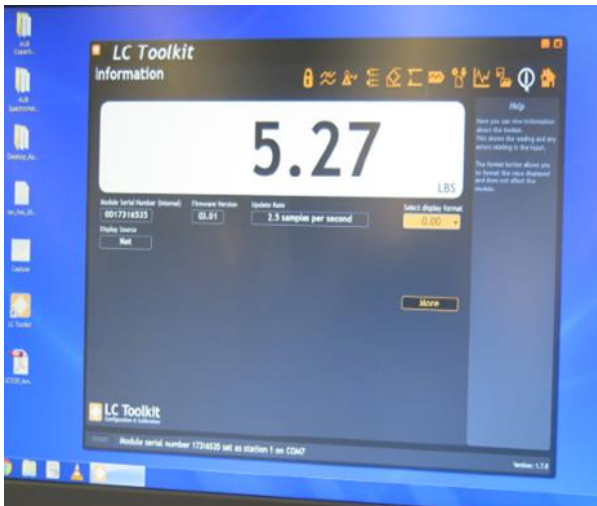
Figure 2 Screen showing load cell measurement in pounds (left) and Hoist-mounted load cell (right)
