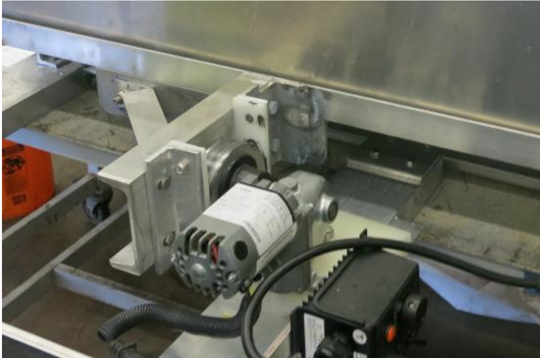
Figure 3 Variable speed motor used to horizontally move the fluid tray and induce surface energy to the test fluid
