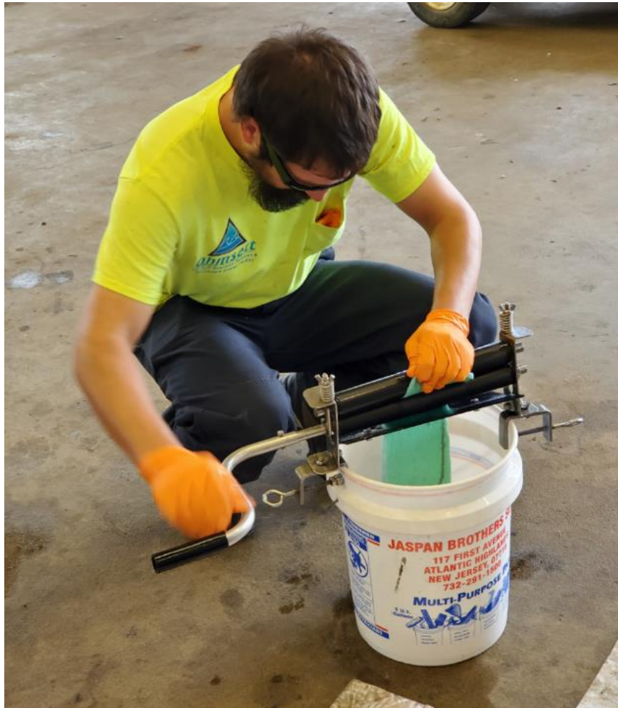
Figure 8 Manual roller system employed for the manual oil recovery tests
