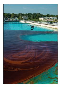
A rotocraft equipped with a thermal infrared sensor captured images of emulsified oil to validate the sensor's capabilities during the NOAA and BSEE funded remote sensing test. mobile platforms at Ohmsett. The study was to compare and determine how well each of the systems detects, monitors, and measures oil slicks and emulsions in the marine environment.
