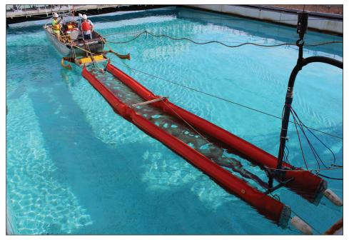
The autonomous skimmer, outfitted with oil thickness sensors, undergoes performance evaluations in the Ohmsett test basin.
