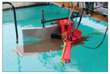
with a universal The MiniBagger is designed with a universal mounting system mounting system en- enabling it to be mounted to small vessels.
