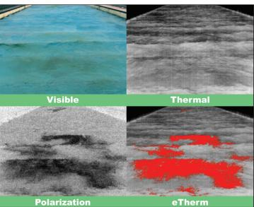
"The Pyxis consistently showed superior detection across all conditions tested and regularly detected oil and diesel in both flat water and breaking waves," said David Chenault, Polaris Sensor Technologies, Inc. President. "A time lapse, overnight test showed the detection performance of the polarization imagery from a factor of 3 to more than 50 times better contrast than standard thermal imaging."
