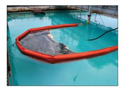
Dispersant treated oil was placed in the apex of the boom to assess the ability of a boom to contain undispersed oil. *ment*, as a guideline, a 50-foot curtain boom was rigged to the main bridge to simulate towing at sea. Oil was preloaded into the apex of the boom which could be monitored in real time using two high definition underwater cameras. The boom was towed at incremental tow speeds to determine when first loss occurred.
