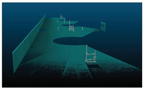
Targets were placed in precise locations in the Ohmsett test basin. The 3D at Depth underwater laser scanning technology scanned the targets to create the above image.
